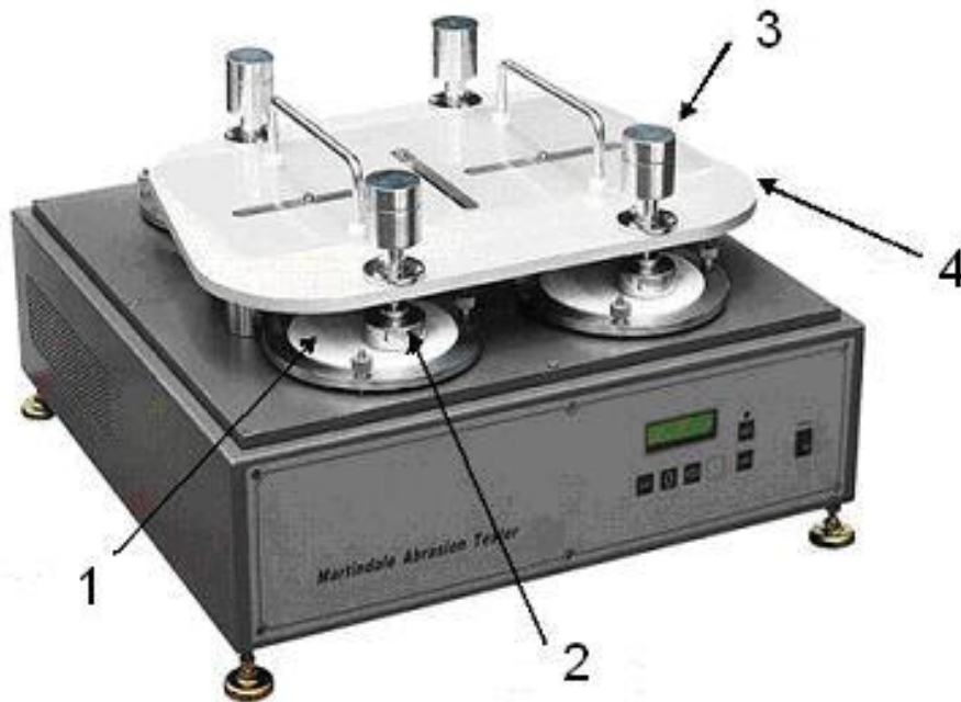
Figure 1 – Layout of the Martindale tester
